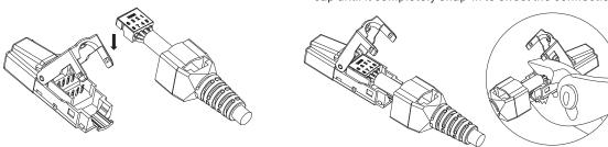
Close plug cover, make sure the drain wire is in proper contact with grounding clip on plug. Pull back strain relief boot to cover the plug, fasten supplied cable tie to secure grounding contact.
