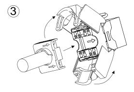
Install the termination cap to outlet, which will also allocate the conductors sitting on the slots.
