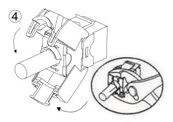
Secure the hinged outlet by using a crimp tool until it completely snap to effect the connection.
