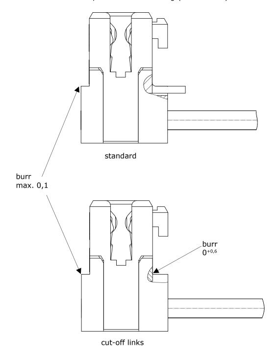
Make sure that the cut-off links do not adhere to the component and that they do not remain in the connector after they are cut off.
