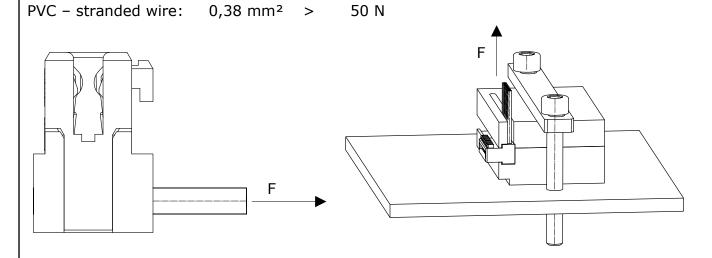
The stated value for the wire pull-out force is a typical value, established during a test with a standard 0,38 mm<sup>2</sup> wire. All values were determined under laboratory conditions and serve as a reference.
