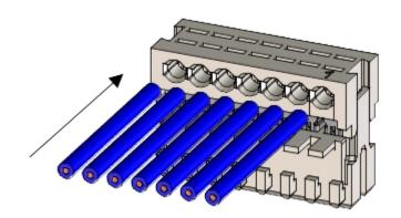
Insulation displacement connection by pressing the top Wire exit  $90^{\circ}$
