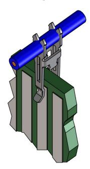
Insulation displacement connection (test acc. to DIN EN 60352-4 / IEC 60352-4)
