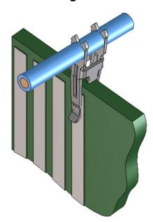
Insulation displacement connection (test acc. to DIN EN 60352-4 / IEC 60352-4)
