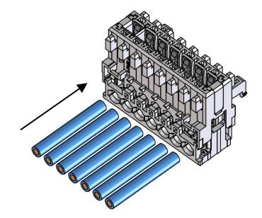
Insulation displacement connection by pressing the top Wire exit  $90^{\circ}$
