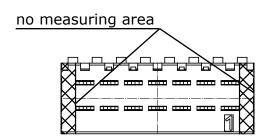
The shut height has to be measured on both sides and in the center area. If a depth gauge is used for measuring, the connector must lay flat with its mating face downwards. A measuring tip of at least  $\emptyset$  3 mm is required. Make sure that the measurement is not distorted by a protruding dovetail guide, pole number marking or similar.
